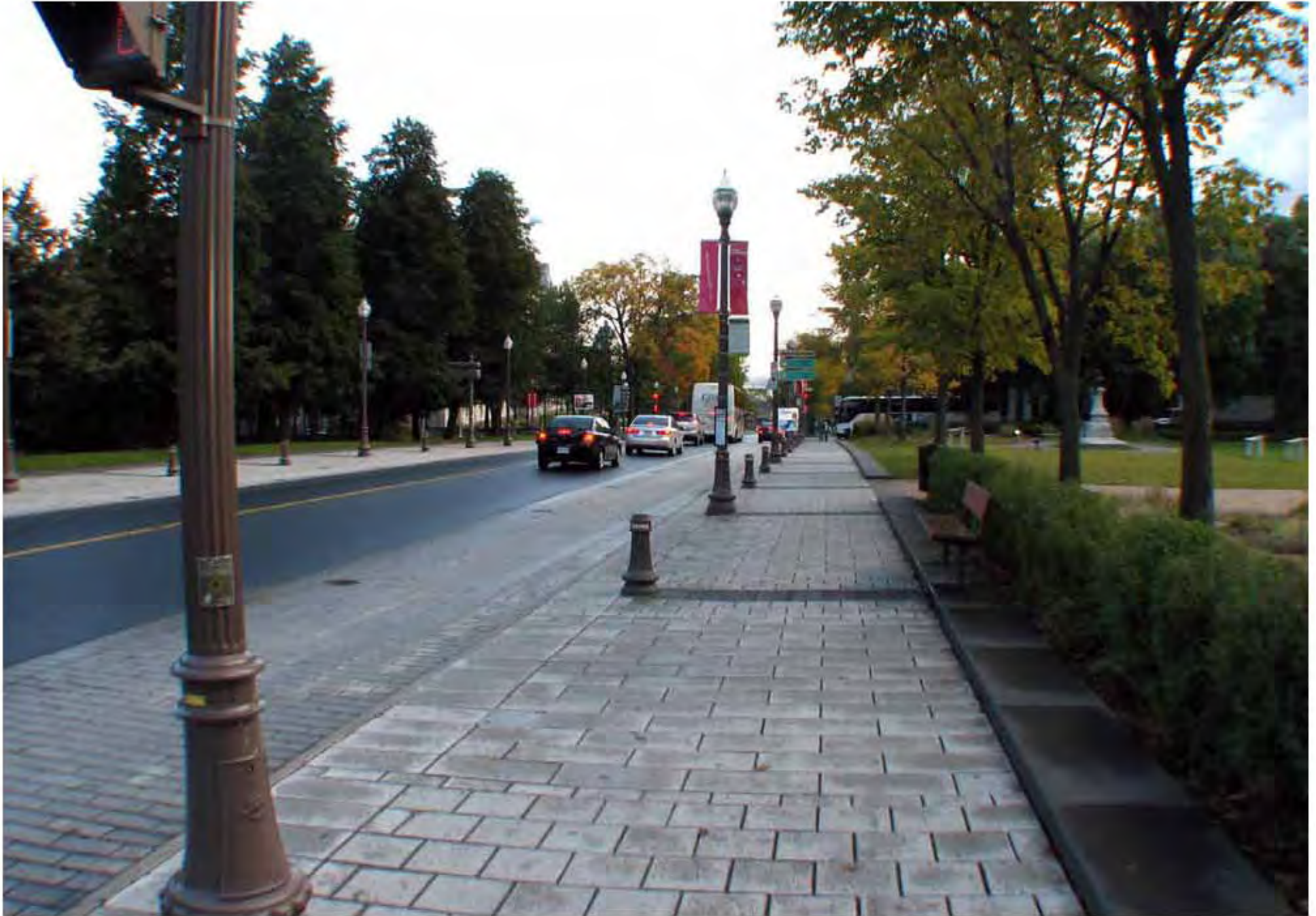
Special pavers along the street to denote on-street parking in Québec City
